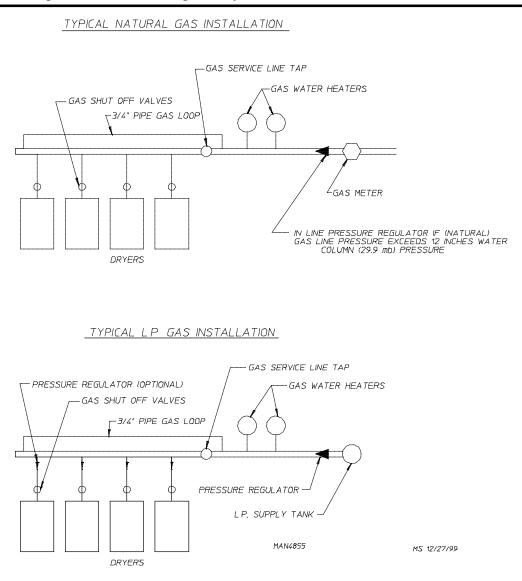
Consistent gas pressure is essential at <u>ALL</u> gas connections. <u>It is recommended</u> that a 3/4-inch (19.05 mm) pipe gas loop be installed in the supply line servicing a bank of dryers. An in-line pressure regulator **must be** installed in the gas supply line (header) if the (natural) gas pressure exceeds 12.0 inches (29.9 mb) of water column (W.C.) pressure.
